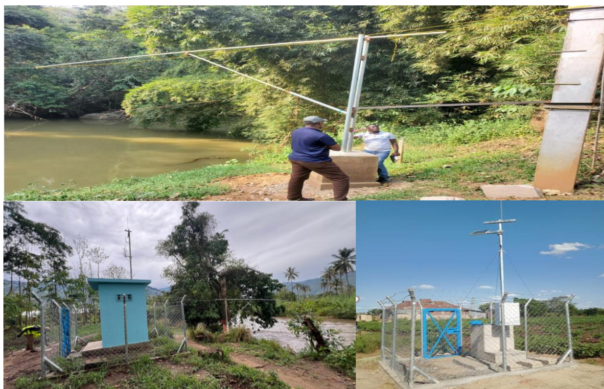
Picture: Diwale at Ngomeno river station installed with Radar Sensor and satellite antenna for sending data and Dakawa GW monitoring station installed with satellite antenna for sending data on real time
