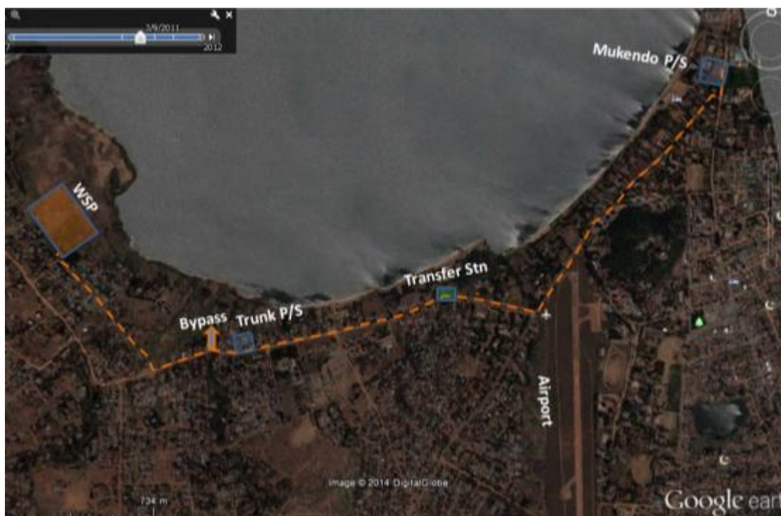
Figure 3: Main sewer from Mukendo pumping station to Makoko WSP.
