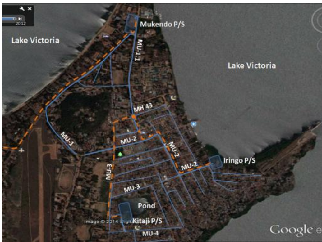
Figure 1: Proposed network of collection sewers in Musoma Municipality Centre
